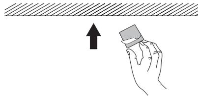
3. After installation, the light is magnetically attach onto the plate and can be easily removed.
