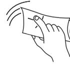
2. Peel off the paper cover of the magnetic installation plates.
