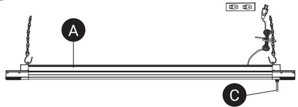
Fold the excess cord and fasten it using a cable tie (not included). Plug power cord into ceiling outlet. The attached pull chain can be lengthened with an additional pull chain (C) if necessary.
