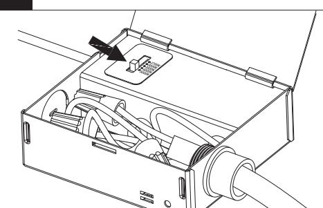
You can choose the light color temperature (from warm white to bright white) with the switch inside the junction box and maintain that light color temperature (fig. 10-11-12-13-14).
