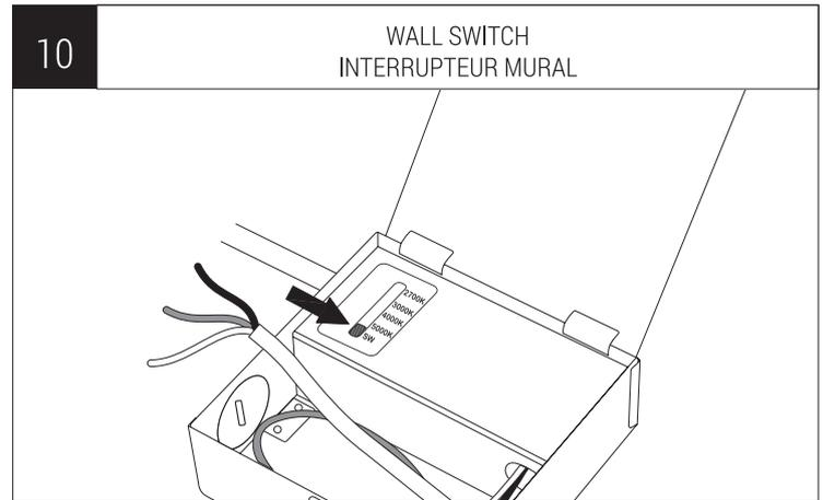
1. You can choose the light color temperature (from warm white to bright white) with the switch inside the junction box and maintain that light color temperature (fig. 6-7-8-9).
